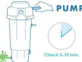
2. Backwash when necessary. Check D.E. filter every 5-10 minutes if water is extremely dirty.
